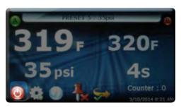
**Note:** When the heat platen is above 100°F (38°C), the current platen temperature is displayed on an orange background as a warning, indicating that the platen is still hot. (2.4)
