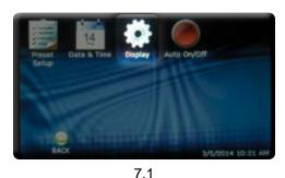
To change your display units, press the Display button in the Setup screen. (7.1)
