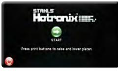
Press and Hold the red Shut Down button until this screen appears. (2.6)
