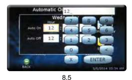
Using the displayed Keypad, enter the numeric time values and press ENTER. (8.5)
